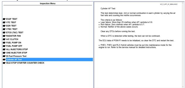
Turn the ignition to OFF then to ON and start the engine according to the screen prompts on the I-HDS. The Cylinder AF Test will begin and will check the performance of injectors 1 through 4 individually.
