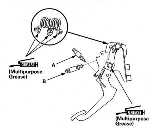
7. Install the clutch pedal assembly (A).
