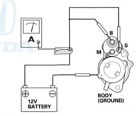
10. If the electric current meets the specification when the battery voltage is at 11.5 V, the starter is working properly.
