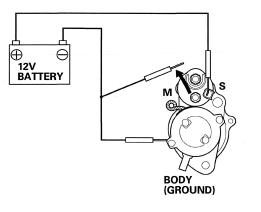
7. Disconnect the battery from the starter body as shown. If the pinion retracts immediately, it is working properly.
