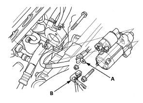
7. Remove the two bolts holding the starter, then remove the starter from under the vehicle.
