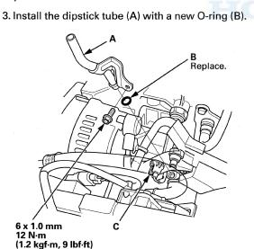
4. Connect the oil pressure switch connector (C).
