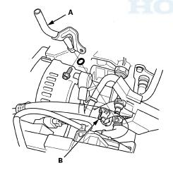
5. Disconnect the oil pressure switch connector (B).
